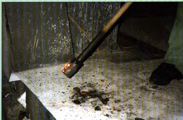
Step 3— The immersion sampler is held in the metal for typically 5 sec. (Times vary according to the thickness of the sample required).
