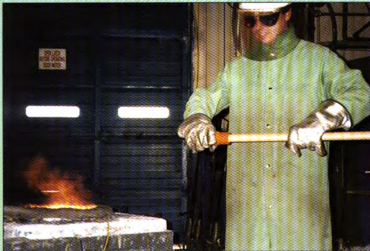
Step 1— The cardboard thermocouple tube is firmly inserted into the sand insert. The tube is then given a quarter twist to lock in place.
