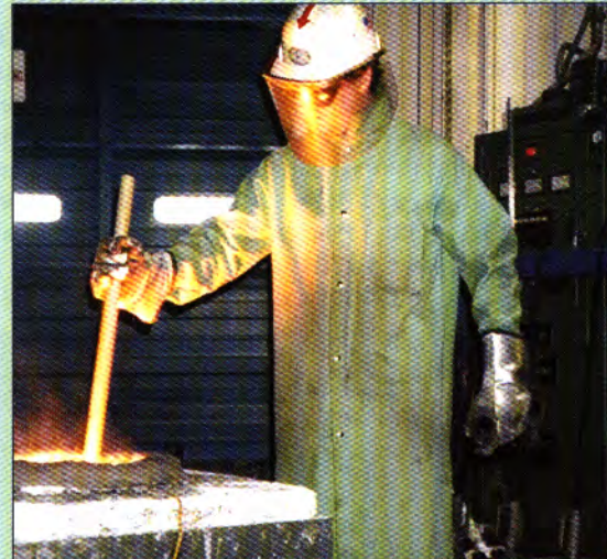
Step 2— The sand insert is immersed into the molten metal. The immersion angle shouldn't be any more than 20° off of vertical to form an accurate sample.
